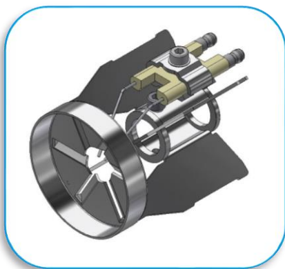
Swirl disk Ø 64 mm for flame tube Ø 80x1,5 mm
